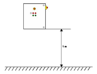
The connecting cables between the control panel and the machine must be protected against damage (cable tray, protective sleeve).
